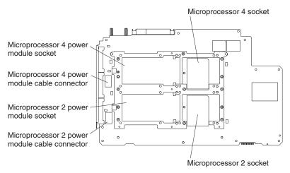
**Important:** To ensure proper server operation after you install replacement or additional microprocessors, install only microprocessors that have the same cache size and type and the same clock speed. For a list of microprocessors supported by your server, go to the ServerProven list at http://www.ibm.com/pc/us/compat/ on the World Wide Web.
